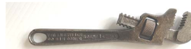
Lawson USHCO Mfg. Co., 6-inch adjustable pipe wrench (BRHS Collection, donated by Mark Zauner)
